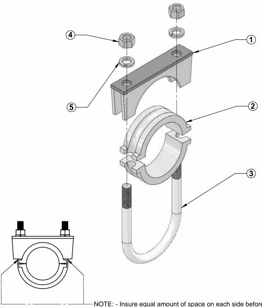
NOTE: - Insure equal amount of space on each side before tightening U-Bolts .
